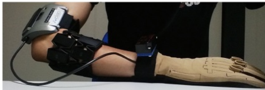
Figure 2.2: Acquisition setup for DB5 using Double Myo
